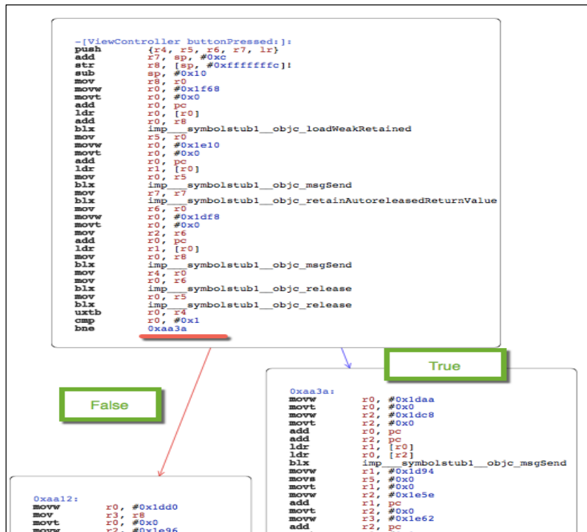
Figure 15. Analysis of control flow graph for Email Button Clicked method
